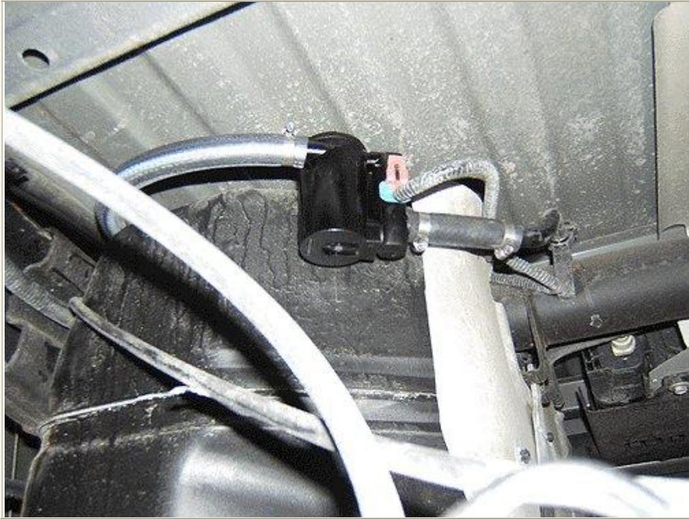
6. Install the new canister vent valve solenoid to the fuel tank clip or mounting bracket as shown above. The valve port closest to the electrical connector must point towards the canister.
