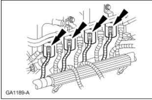
9. Disconnect the eight fuel injector electrical connectors.
