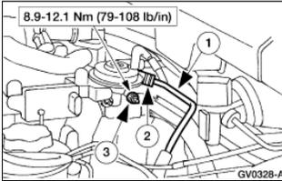
13. Connect the water heater inlet tube hose.
