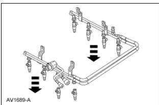
21. Inspect the two O-ring seals from each fuel injector. Install new O-ring seals as needed.
