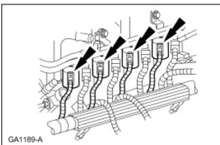
16. Connect the fuel lines. For additional information, refer to [Section 310-00A](#).
