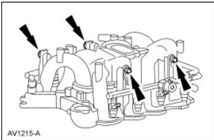
20. Remove the fuel injectors from the fuel injection supply manifold.
