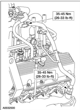
8. Connect the differential pressure feedback EGR transducer electrical connector.
