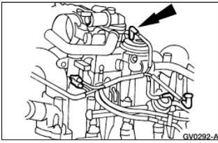
6. Position EGR tube on the engine.
