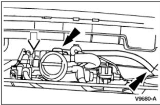
19. Remove the bolts and lift the fuel injection supply manifold (9F792) and injectors upward, out of the intake manifold (9424).
