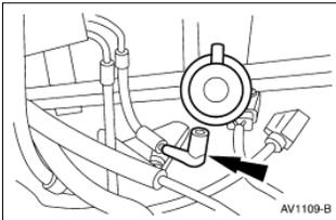
7. **⚠ CAUTION:** After disconnecting, plug the fuel lines to prevent leakage.
