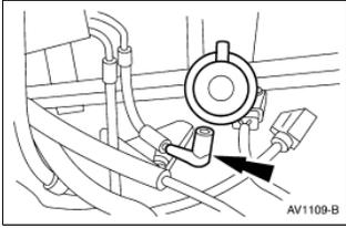
18. Install the accelerator control splash shield.
