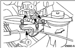
5. Remove the accelerator control splash shield.
