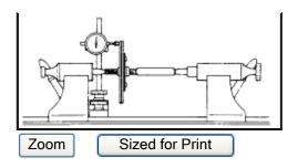
2. INSPECT <u>CLUTCH DISC</u> RUNOUT Using a dial indicator, check the disc runout. Maximum runout: **0.8 mm (0.031 inch)** If necessary, replace the clutch disc runout.
