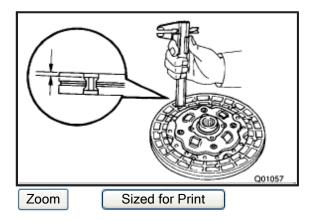
1. INSPECT <u>CLUTCH DISC</u> FOR WEAR OR DAMAGE Using vernier calipers, measure the rivet head depth. Minimum rivet depth: **0.3 mm (0.012 inch)** If necessary, replace the <u>clutch disc</u>.
