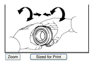
5. INSPECT RELEASE BEARING Turn the bearing by hand while applying force in the axial direction. **HINT:** The bearing is permanently lubricated and requires no cleaning or lubrication. If necessary, replace the release bearing.
