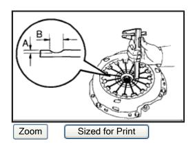
4. INSPECT DIAPHRAGM SPRING FOR WEAR Using vernier calipers, measure the diaphragm spring for depth and width of wear. Maximum: A (Depth): **0.5 mm (0.020 inch)** B (Width): **6.0 mm (0.236 inch)** If necessary, replace the clutch cover.
