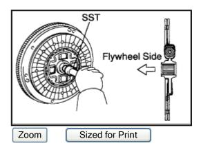
a. Insert SST in the <u>clutch disc</u>, then insert them in the <u>flywheel</u>. SST 09301-00210 **HINT**: Take care not to insert <u>clutch disc</u> in the wrong direction.
