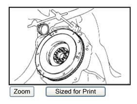
3. INSPECT FLYWHEEL RUNOUT Using a dial indicator, check the flywheel runout. Maximum runout: **0.1 mm (0.004 inch)** If necessary, replace the flywheel. Torque: 1st: **49 Nm (00 kgf-cm, 36 ft. lbs.)** 2nd: Turn **90°**
