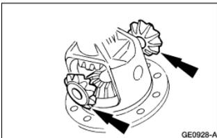
5. Rotate the differential pinion gears to align the differential pinion shaft bore.
