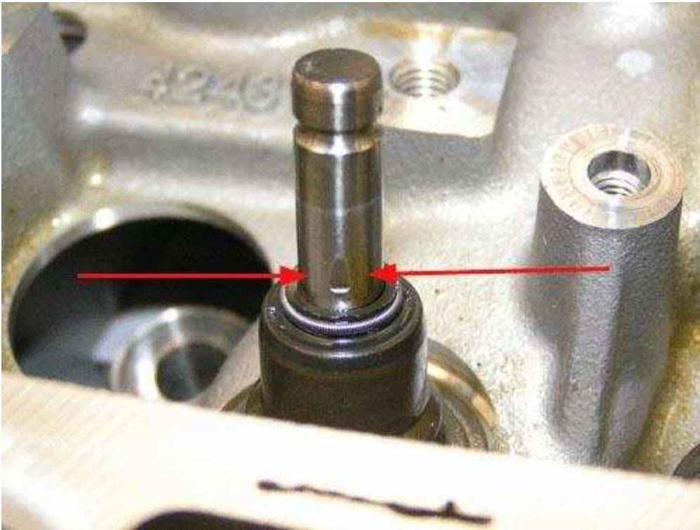
Fig. 2: View Of Nicked Valve Stem (2 Of 2) Courtesy of GENERAL MOTORS CORP.
