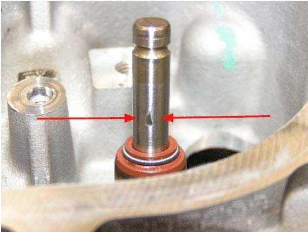
Fig. 1: View Of Nicked Valve Stem (1 Of 2) Courtesy of GENERAL MOTORS CORP.
