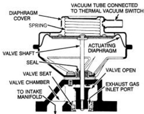
Fig. 1: Cutaway view of a common EGR valve
