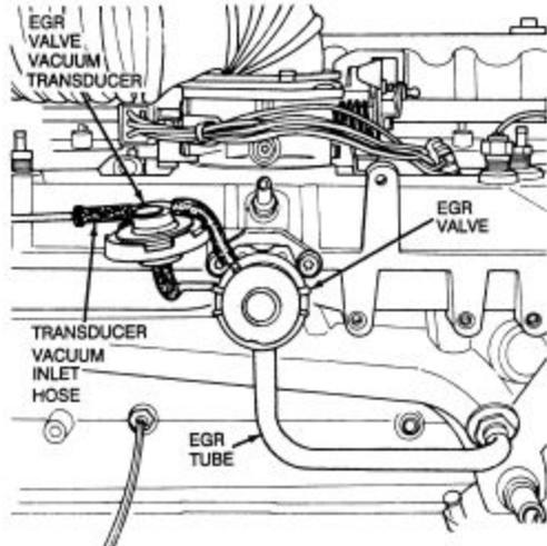
Fig. 3: View of a 4.0L engine with an EGR valve and a vacuum transducer
