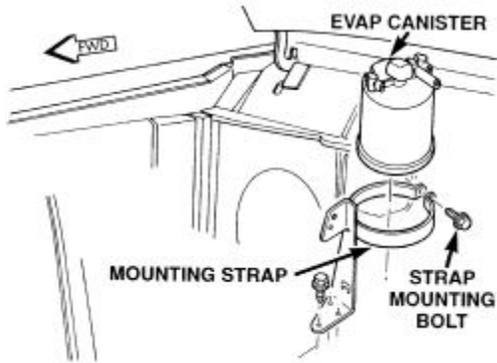
Fig. 1: Exploded view of the EVAP cannister and related components-1996 Cherokee model shown
