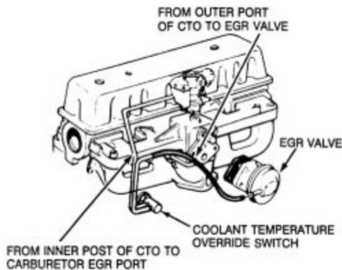
Fig. 5: EGR system using a coolant temperature override switch
