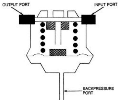
Fig. 4: Vacuum transducer port identification
