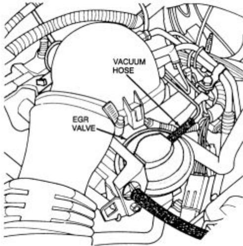
Fig. 6: View of the 2.5L engine EGR valve location
