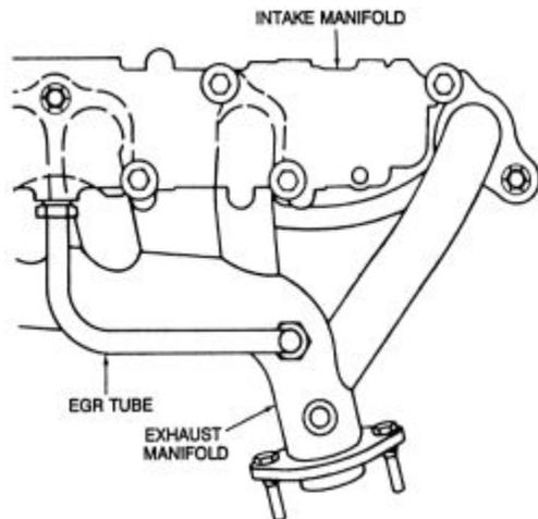
Fig. 10: View of the 4.0L engine EGR tube
