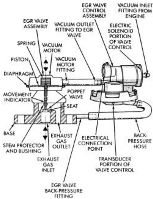
Fig. 11: View of the EGR system and related components-1995 5.2L Grand Cherokee model shown
