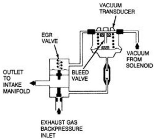
Fig. 2: EGR system with a vacuum transducer
