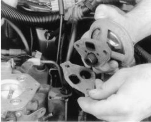
Fig. 8: Remove and discard the old EGR valve gasket
