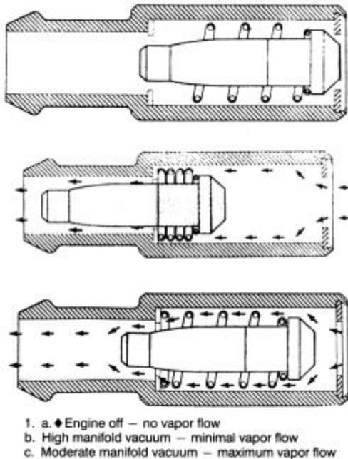
Fig. 1: View of common PCV valve operation
