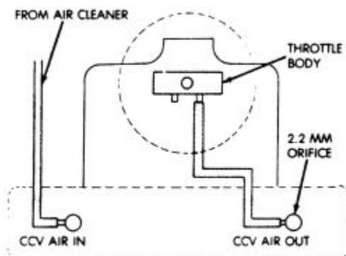
Fig. 3: CCV system diagram for the 2.5L engine
