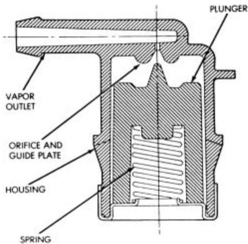
Fig. 5: Cutaway view of the pressure relief/rollover valve
