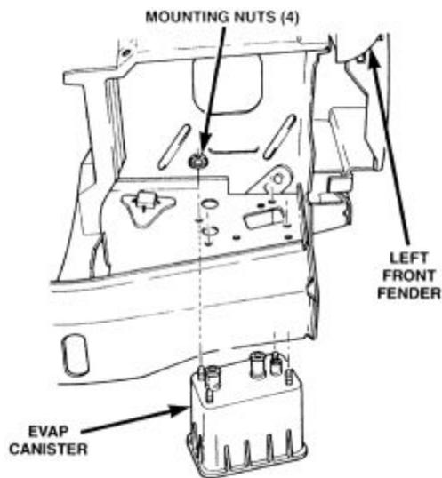
Fig. 2: Exploded view of the cannister location for the 4.0L California emission package-1996 Grand Cherokee model
