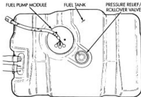
Fig. 6: View of the pressure relief/rollover valve location
