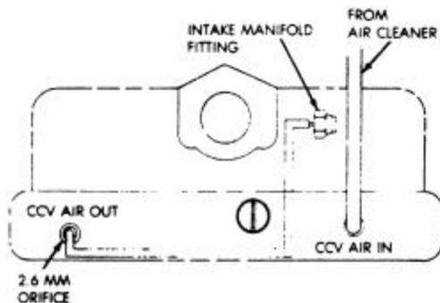
Fig. 2: CCV system diagram for 4.0L engine
