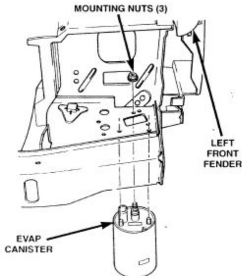
Fig. 3: Exploded view of the cannister location except the California emission package-1996 Grand Cherokee model
