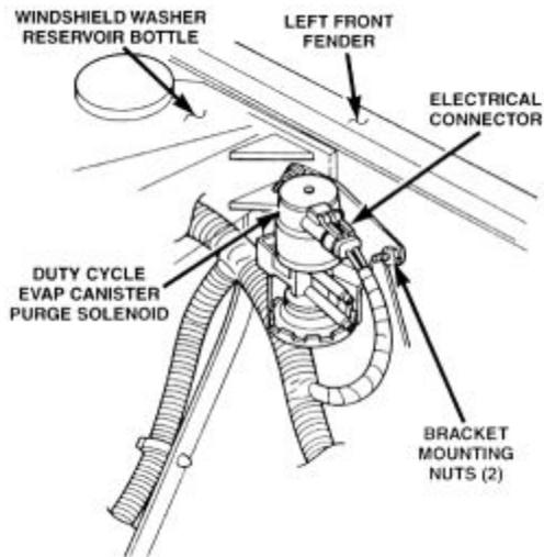
Fig. 4: Common EVAP canister purge solenoid and related components
