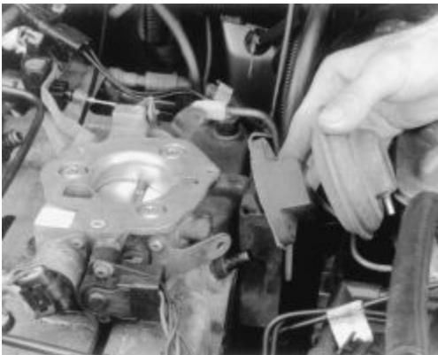
Fig. 7: Removing the EGR valve
