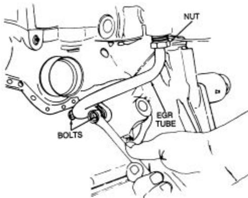
Fig. 9: View of the 2.5L engine EGR tube
