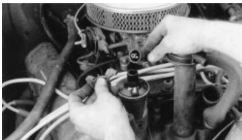
Fig. 1: Disconnecting the wiring from the coil
