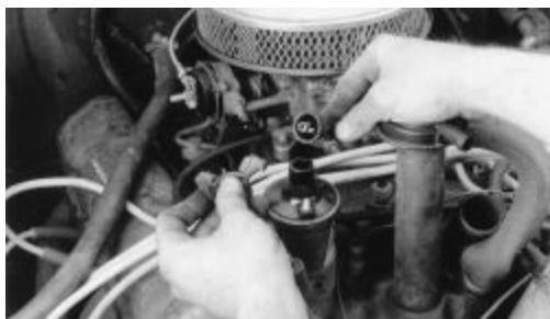
Fig. 1: Disconnecting the wiring from the coil
