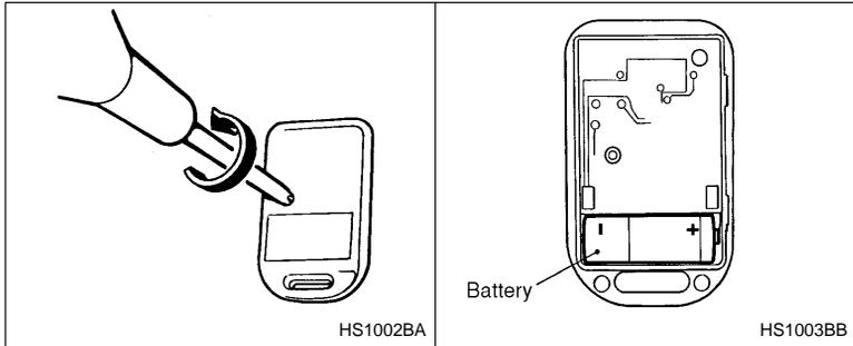
1. Remove the phillips screw on the back of the remote transmitter case. Use a small coin to separate the case halves and expose the battery.
