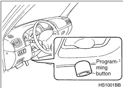
**The Programming Button is located under the driver's side dash beneath the diagnostic connector.**
