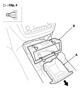
4. Detach the clips and release the hooks (A), then remove the driver's console side trim (B) and passenger's console side trim (C).
