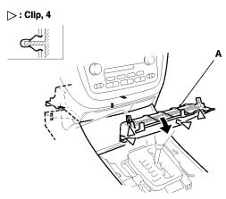
3. With rear entertainment system: Remove the coin pocket (A). Pull the DVD panel (B) out to detach the clips, then remove the panel.
