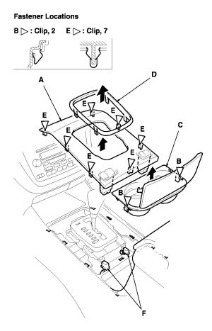
2. Without rear entertainment system: Detach the clips by hand, and remove the center panel lower trim (A).
