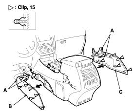
5. Gently pull out the console rear trim (A) to detach the clips and to release the hooks (B), then disconnect the rear heater-A/C passenger's control panel-unit connector (C).
