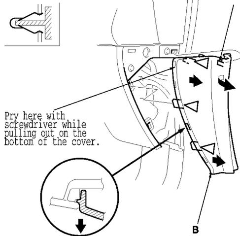
6. Remove the screws (A and B), and detach the clips (C and D). Disconnect the trunk lid opener main switch connector (E) and glove box light bulb socket (F), then remove the glove box cover (G).
