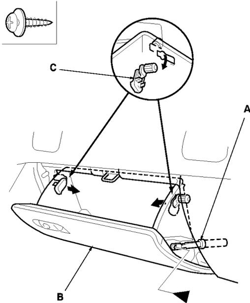
3. Remove the screws, then remove the glove box.
