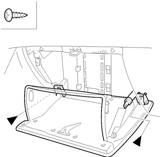
4. Remove the passenger's front console cover.
