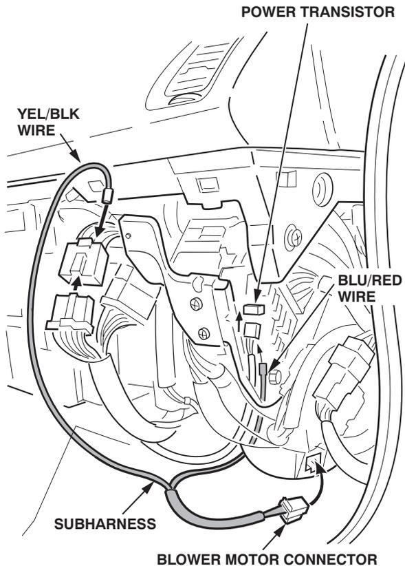
6. Reconnect connector C202 and the power transistor connector, then connect the 2P connector on the new subharness to the blower motor.
