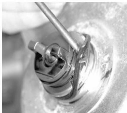
Fig. Use a small pick to remove the O-ring from the distributor
