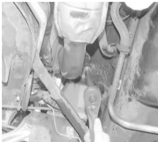
Fig. Fig. 10: With the exhaust system supported with jackstands, unfasten the exhaust pipe flange-to-manifold nuts
