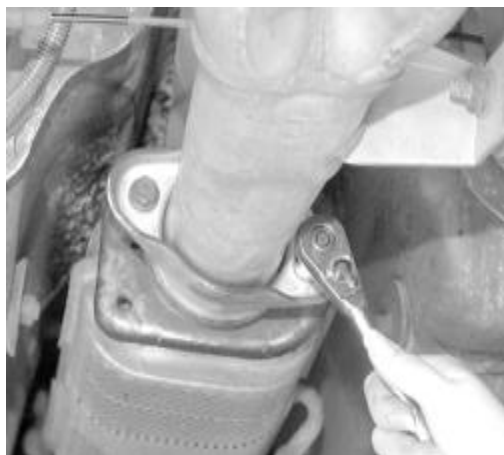
Fig. Fig. 4: On some vehicles, it will be necessary to unfasten the exhaust pipe-to-catalytic converter attaching bolts
