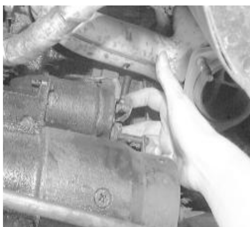
Fig. Fig. 13: ...then pull the wiring off of the stud
