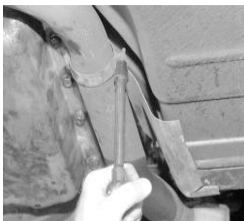
Fig. Fig. 5: Unfasten the exhaust pipe clamp retaining bolts
