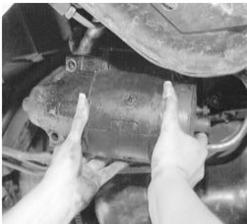
Fig. Fig. 16: Be careful when lowering the starter, because it is heavier than it looks!
