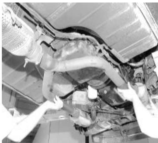
Fig. Fig. 11: With the help of at least one assistant, carefully lower the exhaust and place in a safe place
