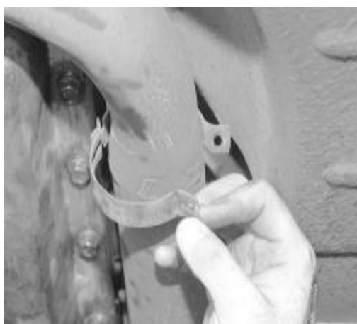
Fig. Fig. 6: Then, unfasten the clamp from the exhaust pipe
