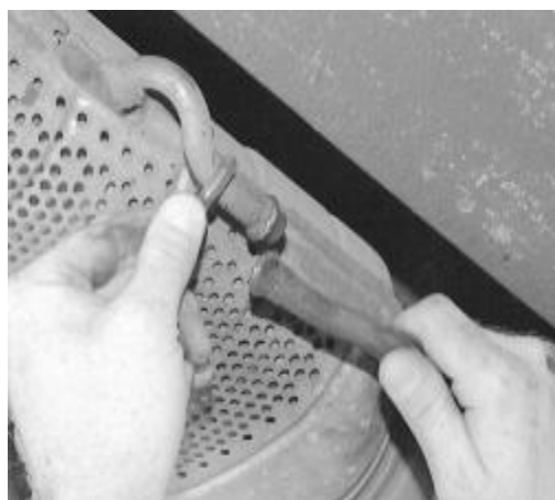
Fig. Fig. 8: Then move the clamp aside and separate the converter air pipe for exhaust removal
