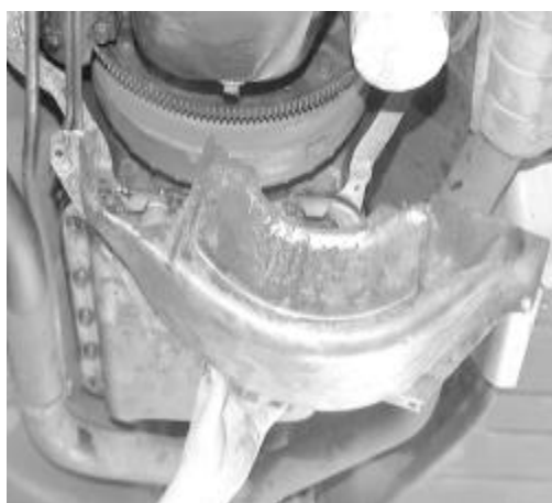
Fig. Fig. 3: Remove the bolts, then lower the flywheel cover. It will probably take some maneuvering to get the cover out
