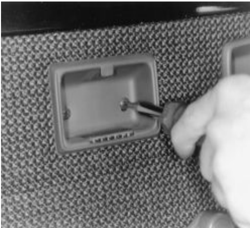
Fig. Fig. 10: ... and remove the retainer screws securing the ashtray holder assembly
