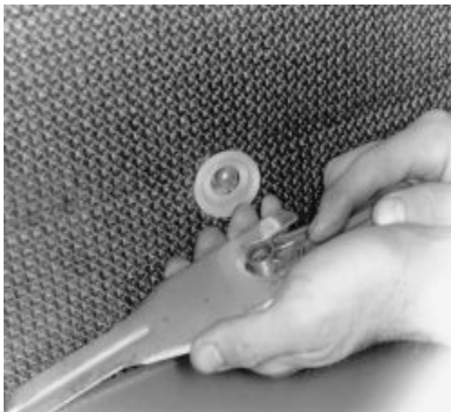
Fig. Fig. 14: ... to separate the crank from the window regulator stud
