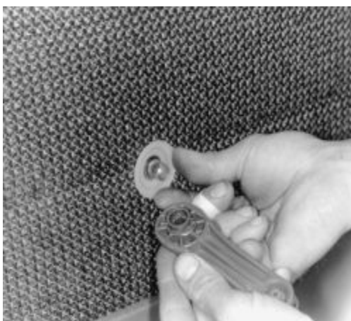
Fig. Fig. 15: Insert the crank arm clip to the crank, and remove the washer, then place the pieces aside
