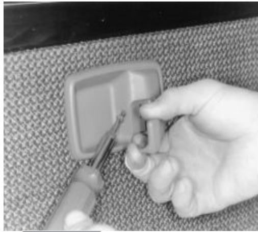
Fig. Fig. 12: Remove the door handle trim panel retainer screw
