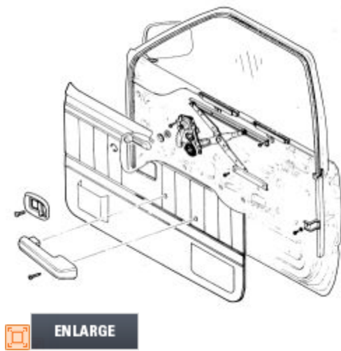
Fig. Fig. 2: Door and panel assembly—later model Pick-up shown (other late models similar)
