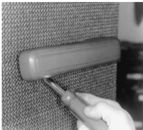
Fig. Fig. 7: Remove the retainer screws from the bottom of the armrest-1986 Trooper shown
