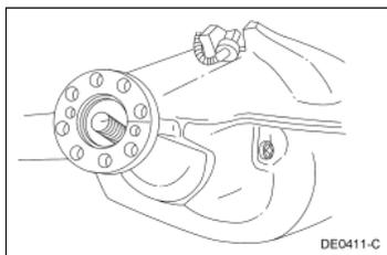
5. Using the special tool, install the pinion flange.
