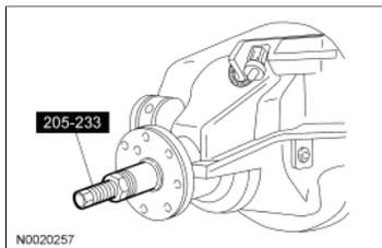
6. **CAUTION:** Install a new pinion nut with the same color as the original if not replacing the collapsible spacer. If a new collapsible spacer is installed, install the nut in the kit, as indicated in the chart below, or damage to the component may occur.
