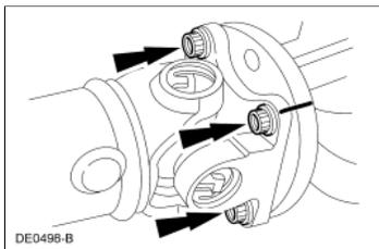
5. **NOTE:** The driveshaft centering socket yoke fits tightly on the pinion flange pilot. Never hammer on the driveshaft or any of its components to disconnect the driveshaft centering socket yoke from the pinion flange. Pry only in the area shown with a suitable tool to disconnect the driveshaft centering socket yoke from the pinion flange.
