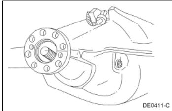
9. Using the special tool, remove the pinion flange.
