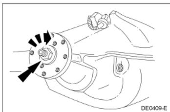
7. Using the special tool to hold the pinion flange, remove and discard the pinion nut.
