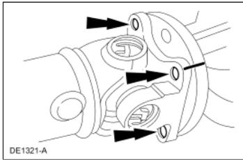
9. **NOTE:** The driveshaft centering socket yoke fits tightly on the pinion flange pilot. To make sure that the driveshaft centering socket yoke seats squarely on the pinion flange, tighten the driveshaft flange bolts evenly in a cross pattern.
