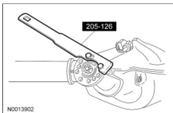
8. Position the driveshaft and align the index mark on the pinion flange.
