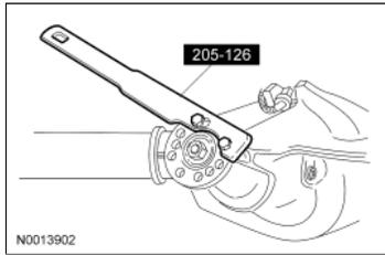
8. Index-mark the pinion flange in relation to the drive pinion stem to make sure of correct alignment during installation.
