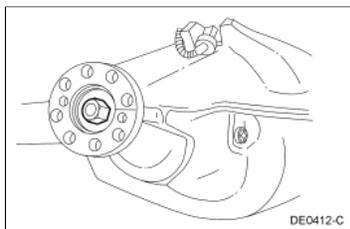
7. **CAUTION:** Under no circumstances is the pinion nut to be backed off to reduce drive pinion bearing preload. If reduced drive pinion bearing preload is required, a new drive pinion collapsible spacer and pinion nut must be installed or damage to the component may occur.
