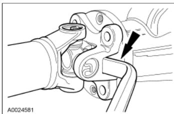
6. Using a Nm (lb-in) torque wrench on the pinion nut, record the torque required to maintain rotation of the pinion gear through several revolutions.
