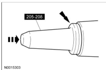
3. Lubricate the pinion flange splines with axle lubricant.
