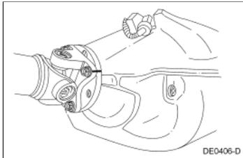
4. Remove the 4 driveshaft flange bolts.
